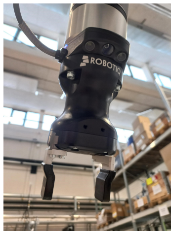
Figure 2: Wrist camera mounted on the UR5e cobot
